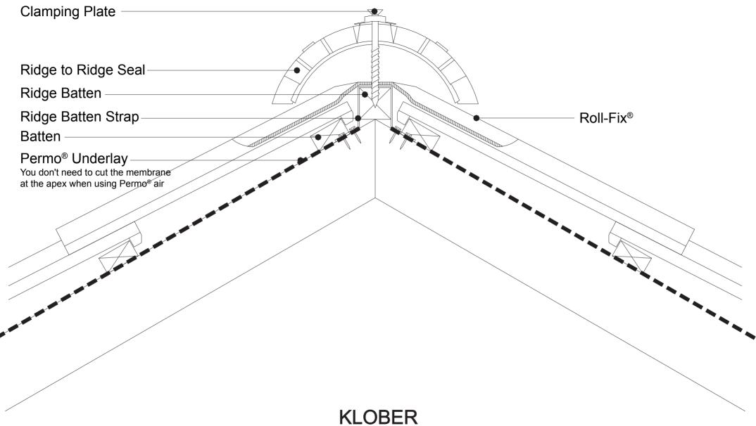
ROLL-FIX® KIT - HALF ROUND RIDGE WITH INTERLOCKING TILES DRG No. KL010
